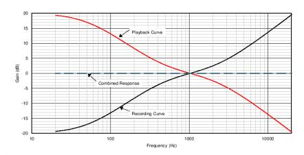
This is called the RIAA curve, and is used when recording onto vinyl. The reason being, if it were normal flat frequency response then you would have very fat grooves for the lower bass frequencies, so this is reduced, and then re-boosted inside the pre-amplifier (mixer).
